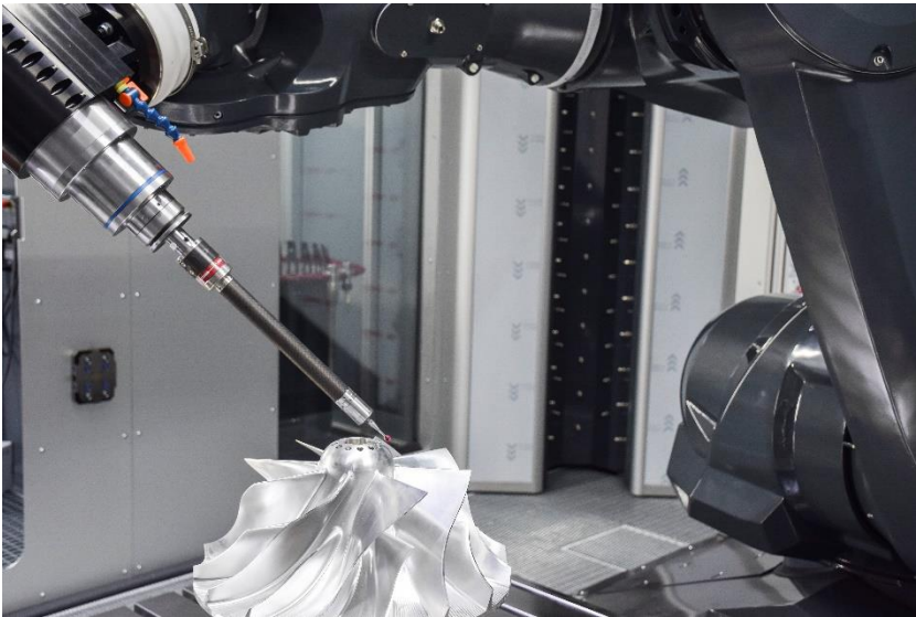
Image 6: Automated measurement in the robot cell - only in this way is it possible to ensure unmanned quality around the clock in the original setup.
