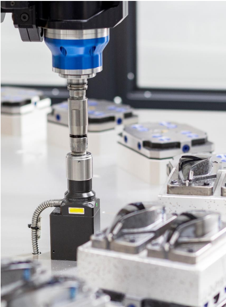
Image 2: The felt tool wears quickly and the Z-Nano tool setting probe therefore measures the current tool length prior to each polishing cycle.
