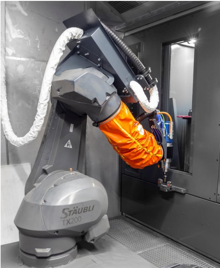
Image 4: Milling precision with the robot arm depends decisively on regular tool measurements using the BLUM laser measuring system.
